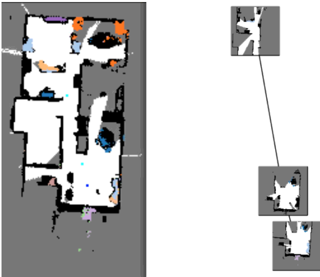
Fig. 1. An example of a TLO2M. The left figure shows the entire O2M map of the trajectory and the right one is the corresponding O2M. The colored grid represents the most major object classes in that position. The cyan dots of the left map corresponds to the node positions of TLO2M of right side. The edges represent the rough relative position of the nodes. The blue dot represent the initial point.
