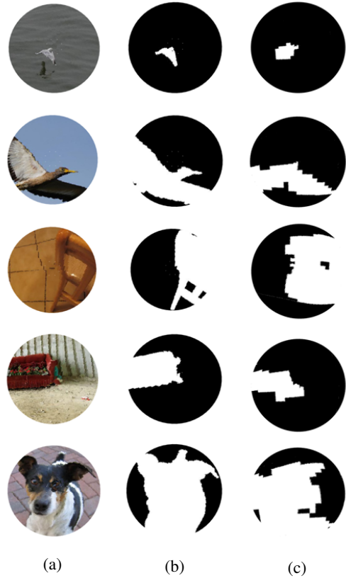
Fig. 10: Some examples of the CEONet results. 441 single eyes of 10 \times 10 pixels are used. (a) PASCAL VOC 2012 images on compound eye camera. (b) Ground-truth maps of (a) in the compound eye data format. (c) Inferred objectness by the CEONet.
